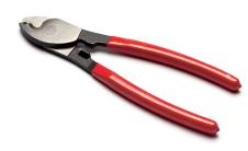
Drop forged steel hand held cutting tool, suitable for stranded non-armoured copper and aluminium cables up to 38mm<sup>2</sup> with two cutting positions (10mm<sup>2</sup> and 38mm<sup>2</sup>).
